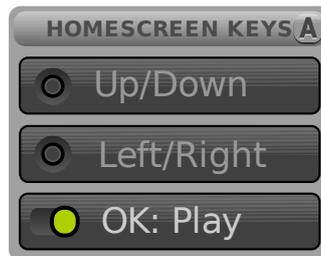
To configure the **OK** button, select the bottom entry and use **LEFT** and **RIGHT** arrow keys to switch between *Menu* and *Play*. The former allows the **OK** button to bring up the menu (default), the latter changes the **OK** button to act as a Play / Pause button in the USB mode.
